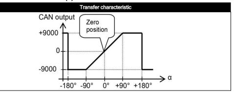
Default 0°: horizontal (label upwards), no acceleration applied. To eliminate mounting offsets the sensor can be zero-ed within ±5° tilt (by the CAN object dictionary)
